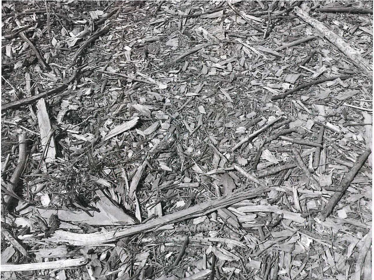
Photo 1029. Lead flakes on Pistol Range floor from bullets flattened by impact on steel targets.
